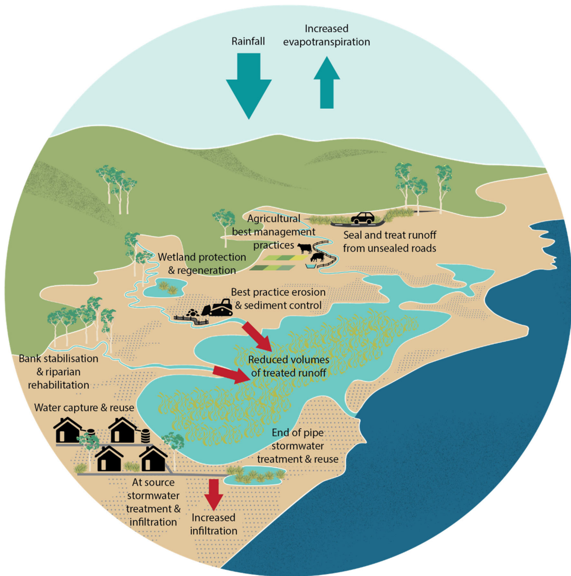
Figure 5-7 Conceptual catchment model – best management practices (adapted with permission from Central Coast Council)
