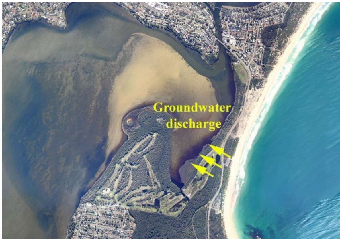
Figure 4-30 Groundwater seepage plumes as evidenced by dark tannin-stained water at Budgewoi
