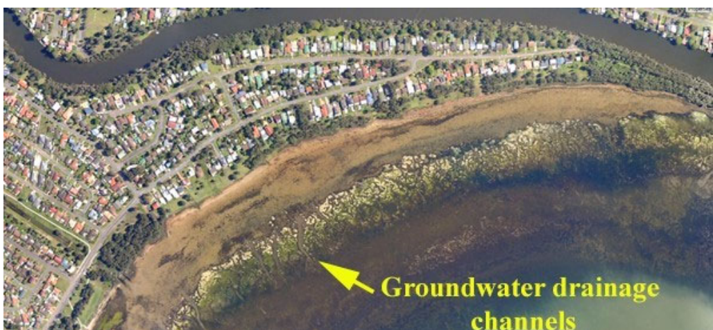
Figure 4-29 Evidence of possible groundwater seepage channels at Chittaway Bay
