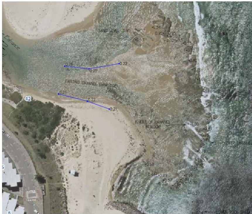
Figure 3-9 Rock shelf elevation and location
