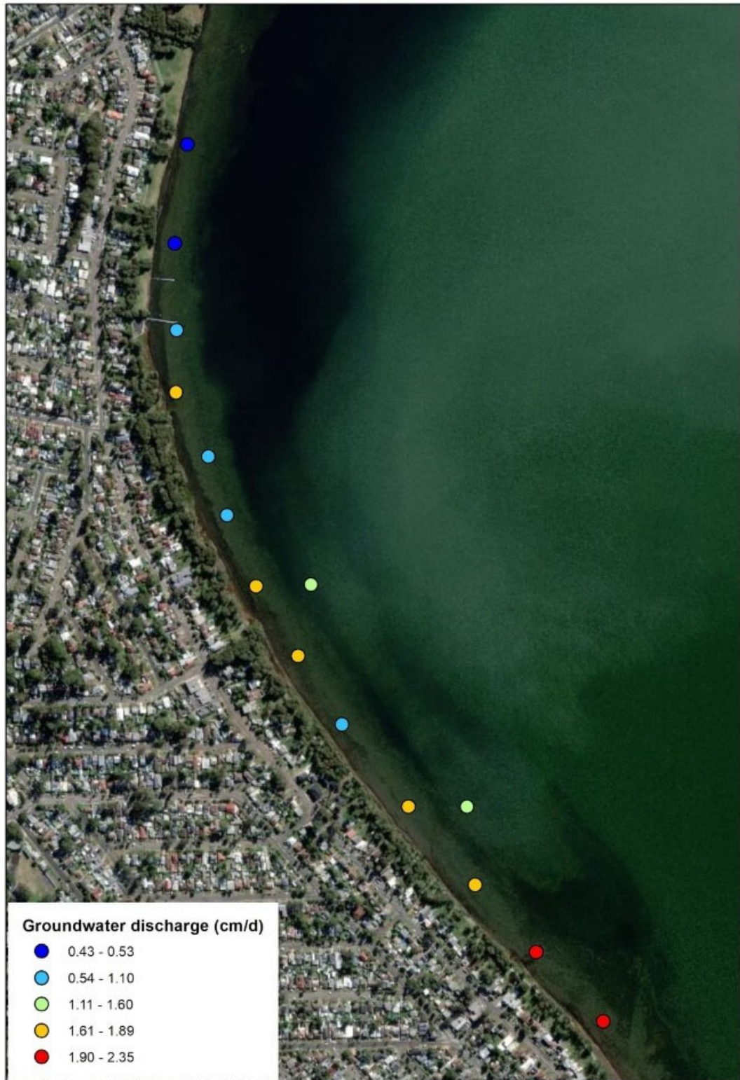
Figure 4-33 Groundwater discharge rates determined along the Berkley Vale shoreline using a natural groundwater tracer technique
