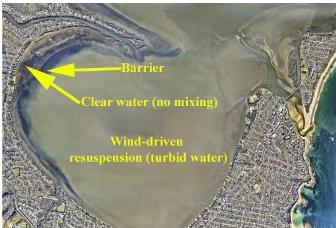
Figure 4-21 Southern Tuggerah Lake during high winds resulting in sediment resuspension
