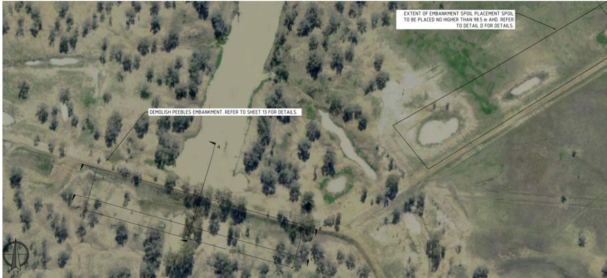
Figure 12 Peebles Dam Location of embankment to be removed and spoil placement (Alluvium Detail Design Drawing 24/08/18)
