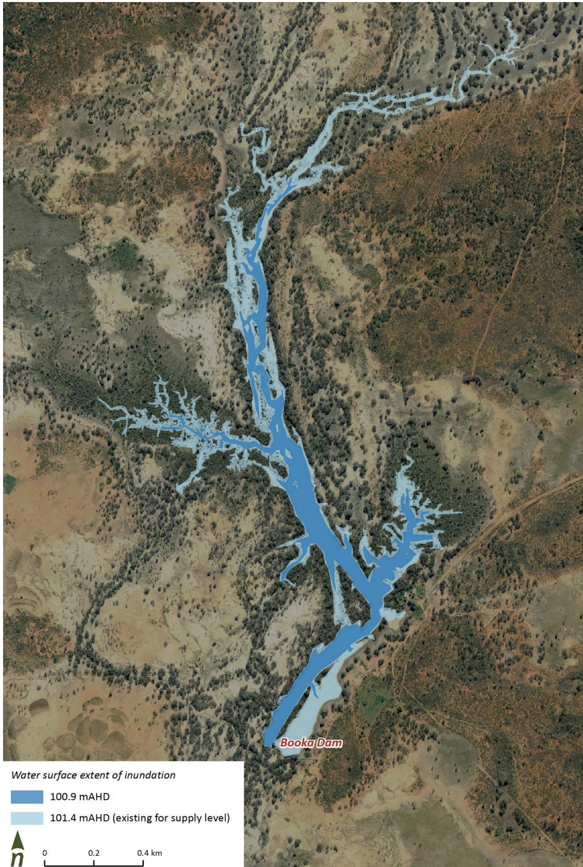
Figure 5-8: Comparison between current full supply level and the proposed full supply level of Booka Dam (Alluvium, 2016)
