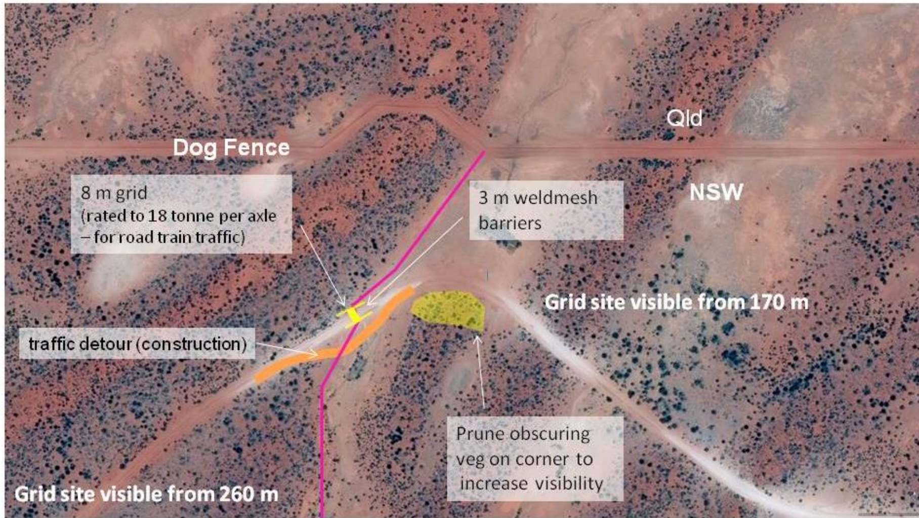
Figure 11: Construction details for proposed grid at intersection of the northern wing fence and Dunes Scenic Drive
