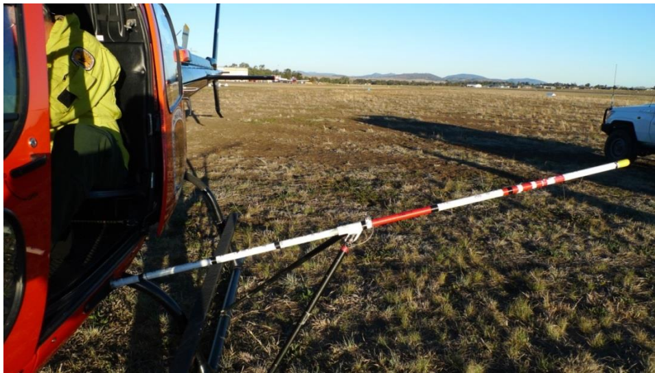
Fig. 9 Distance boom mounted on the left-hand side of the Eurocopter AS350 Écureuil helicopter used in the survey. The distance bins used in the surveys (0-20 m, 20-40 m, 40-70 m, 70-100 m and 100-150 m) are indicated by the black bands on the boom.
