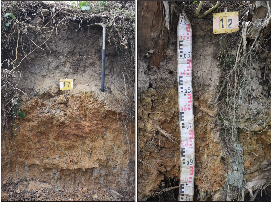
Figures 22 and 23 To left, site 12 (Natric Kurosol), typical of the central drainage plain, showing bleached A2 horizon and poorly drained, mottled clayey B horizon. To right, site 17 (Anthrosol/Brown Sodosol), typical of the surrounding footslopes, showing a deep layer of fill above a bleached A2 and poorly-drained, mottled clayey B horizon. Photos: Mark Young/OEH
