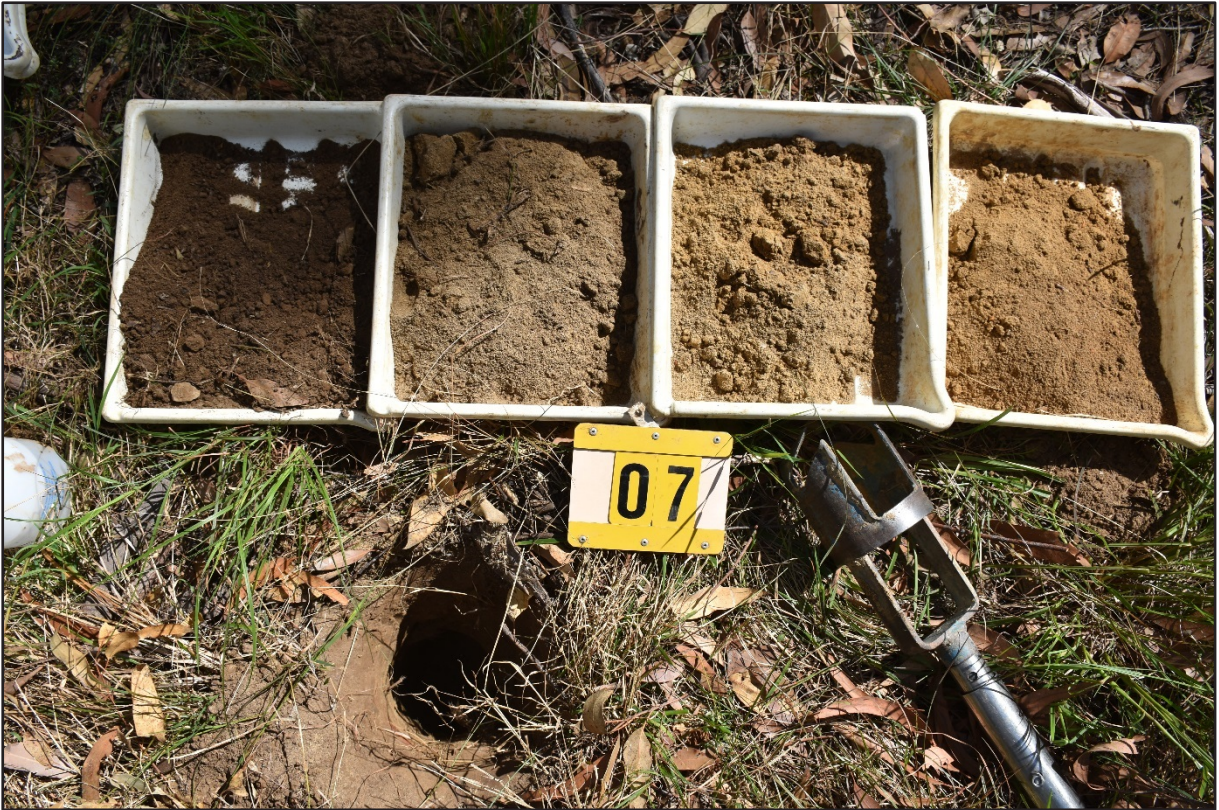
Figure 11 Sandy clay loam topsoils (left) overlying paler A2 horizons (middle) and a clayey sand subsoil (right). Photo: Mark Young/OEH
