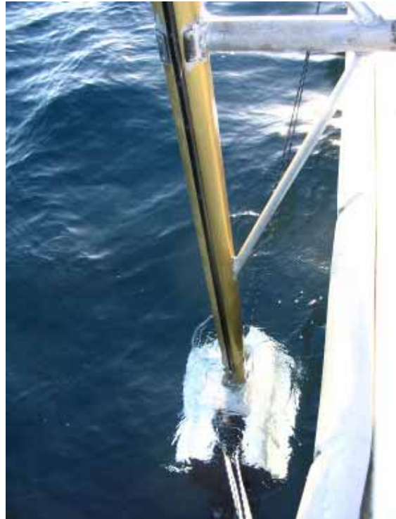
Figure 3. Set up of pole-mounted Geoswath transducers on RV Glaucus .
