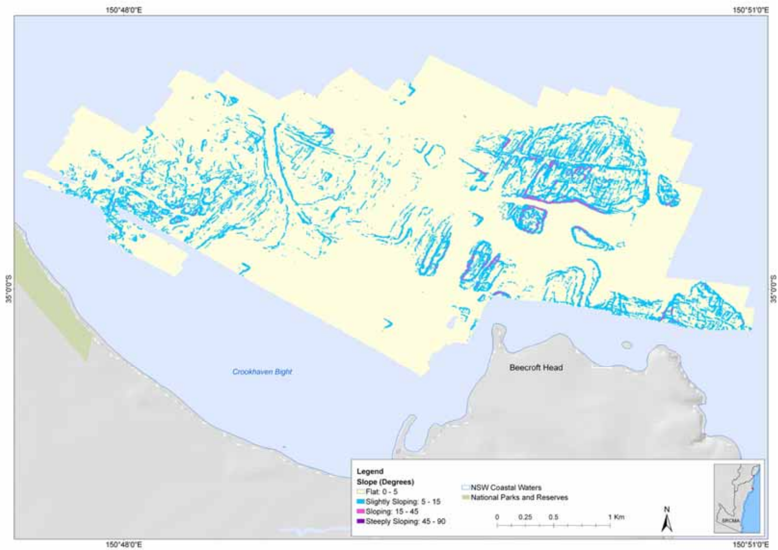
Figure 120. Slope model of the seabed within Crookhaven Bight.
