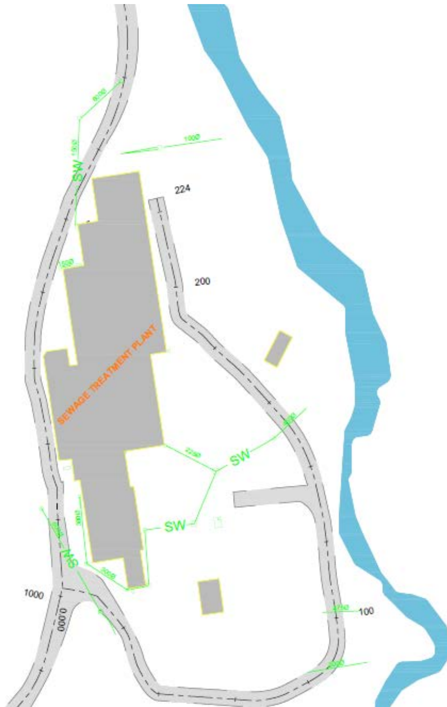
Figure 6 Stormwater drainage network at Perisher Valley Sewage Treatment Plant
