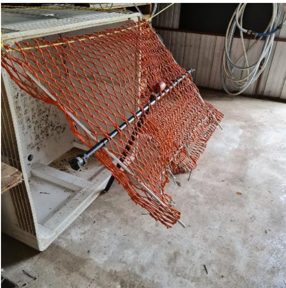
Figure 5-2: Mock-up of a net exclusion barrier as described for the proposed bridge crossings with floats and bracing in the middle of the net to maintain the structure of the excluder and weighted rope at the bottom (Source: Austral Research and Consulting).
