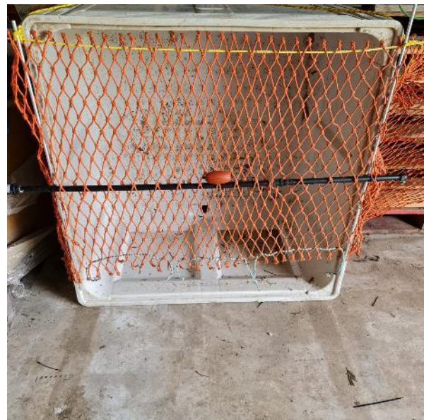
Figure 5-2: Mock-up of a net exclusion barrier as described for the proposed bridge crossings with floats and bracing in the middle of the net to maintain the structure of the excluder and weighted rope at the bottom (Source: Austral Research and Consulting).
