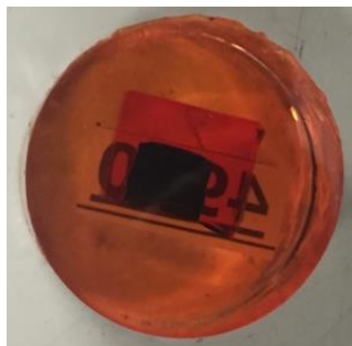
Figure 4. Dust sample in polished polyester resin block
