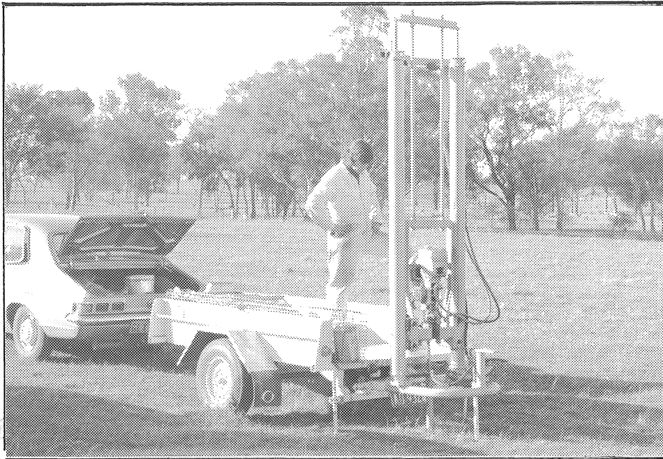
Soils are sampled with a mechanised coring machine.
