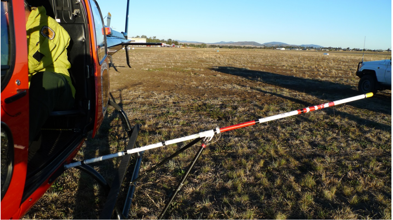
Fig. 5 Distance boom mounted on the left-hand side of the Eurocopter AS350 Écureuil helicopter. The distance bins used in the surveys (0-20 m, 20-40 m, 40-70 m, 70-100 m and 100-150 m) are indicated by the black bands on the boom.
