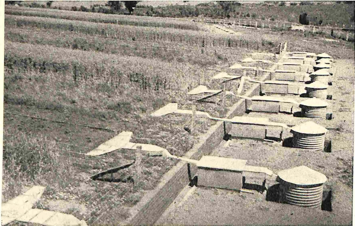
Fig. 2.—Equipment for the collection of run-off from plots on the Cowra Research Station.
