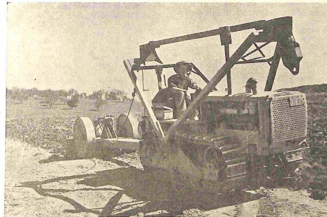
Fig. 2.—A ripper can be used to break up impermeable soil and so improve water penetration.
