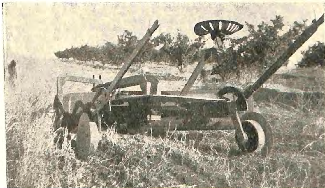
Fig. 2.—The versatile grader ditcher, a useful implement for mechanical soil conservation work.
