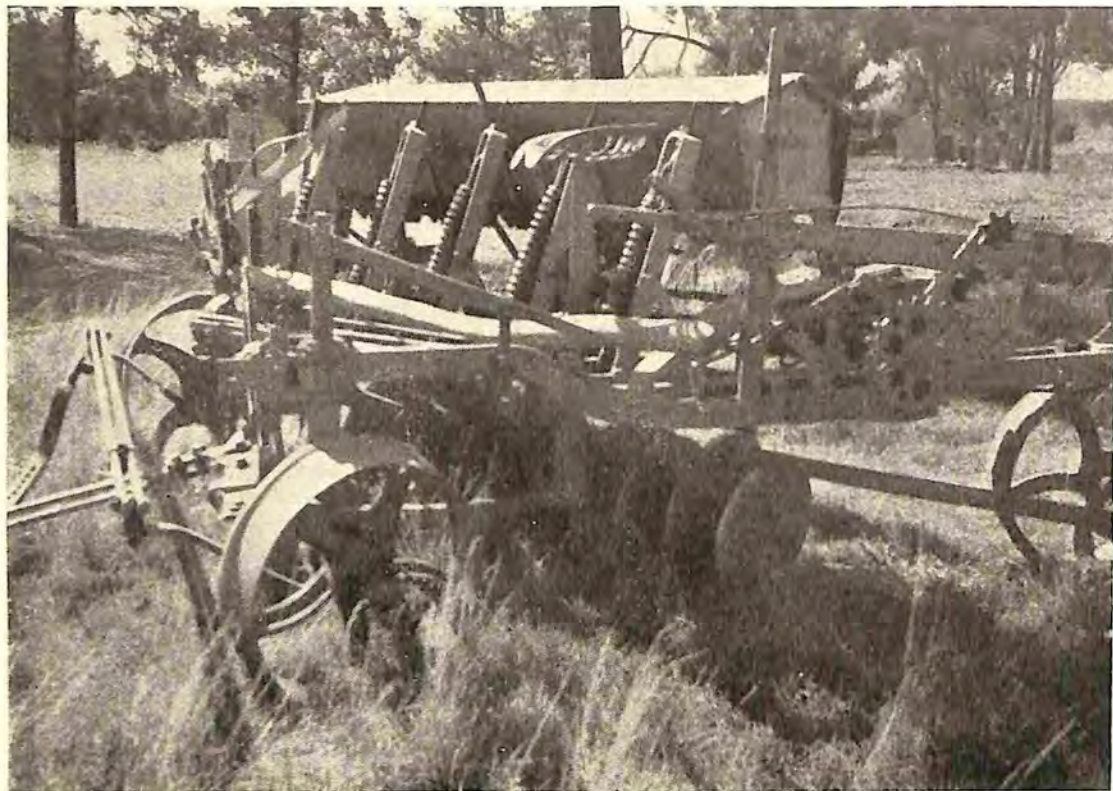
Fig. 5.—A disc plough fitted with seed and fertiliser attachment. An excellent type of implement for stubble farming and pasture establishment.
