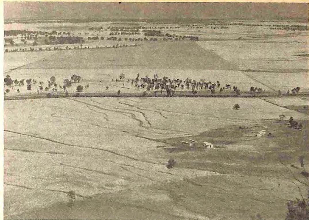
Fig. 3.—This soil is of high detachability and many gullies have developed. A characteristic of these gullies is that they tend to be of about uniform size from top to bottom of slope. This may indicate that the flow is charged to the limit of its transporting capacity all the way from the hill top to valley bottom and the transportation factor limits erosion.
