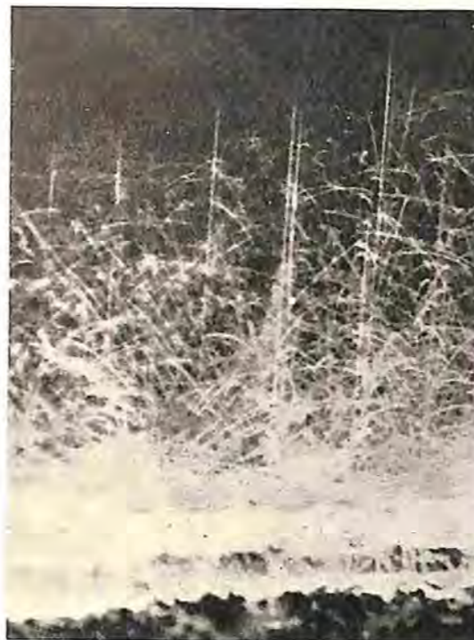
Fig. 3.—This photo. illustrates falling raindrops (the long vertical lines) and splashing particles of soil and water (the curved lines). (Reproduced from "Agricultural Engineering," August, 1947.)
