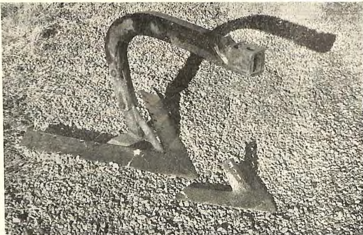
Fig. 3.—Rigid tyne of Dempster carrier fitted with 30 inch sweep with 16 inch sweep on the ground for comparison.
