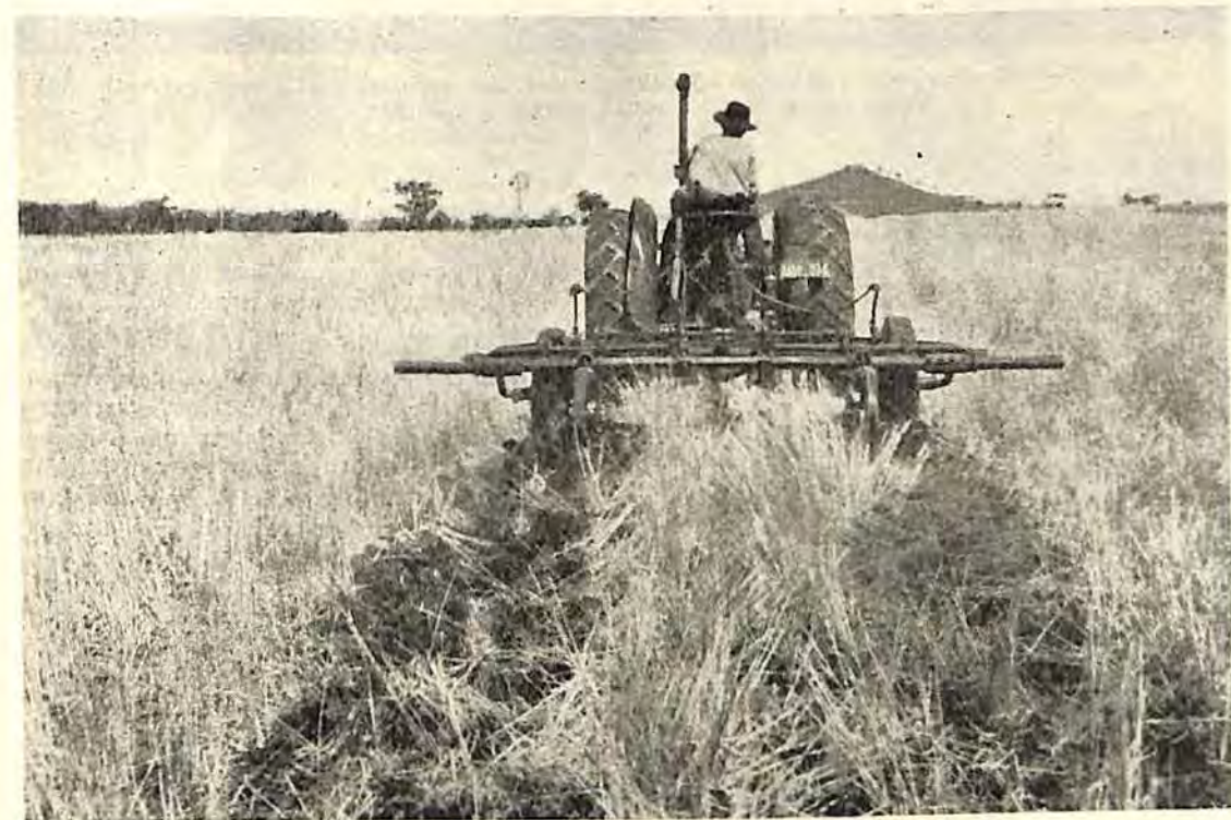
Fig. 6.—Initial cultivation with 30 inch sweeps leaves the surface rough and most of the straw standing.
