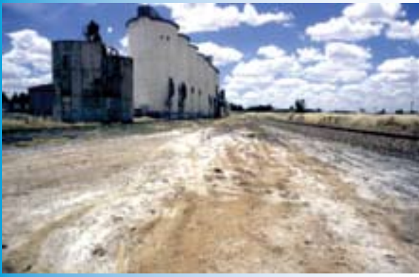
Water movement affected by the railway line has encouraged salt accumulation at the soil surface. Photo: NSW DPI
