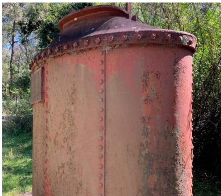
Plate 18: One of the retorts used in the kerosene works (Source: Niche Environment and Heritage)
