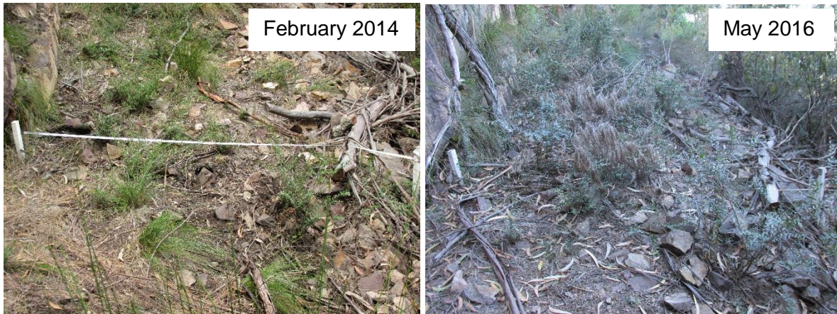
Figure 26: Photo points showing threshold trigger for track depth at site MSB003 Measurements are taken across the track, between two white pegs. February 2014 shows baseline track condition and May 2016 is when the trigger was detected.
