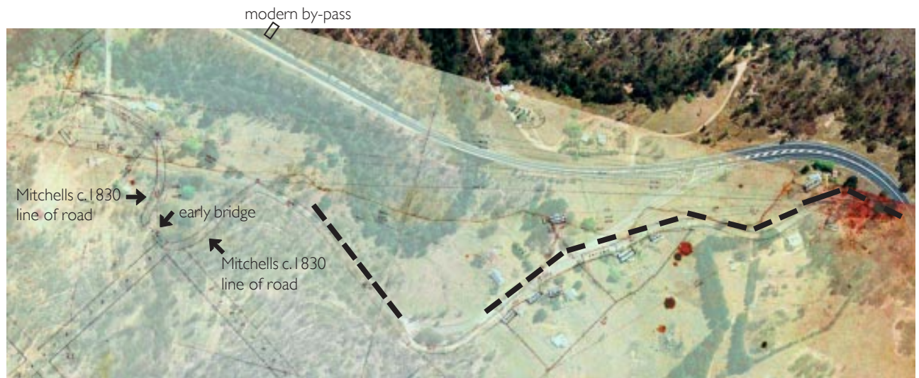
KEY ─────────── Sections of Mitchell's line of road largely retaining their original alignment
