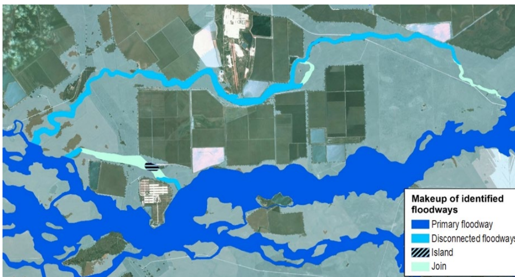
Figure 2 Example of manual edits required when using the indicator technique to meet key requirements of a floodway in rural floodplain management plans
