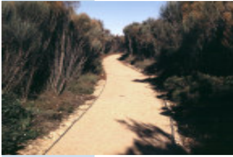
Figure 4.10b Crushed sandstone surface provides disabled access and blends with vegetation.
