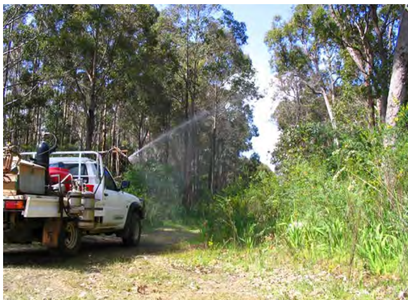
Vehicle-mounted spray rig suitable for high volume spraying
