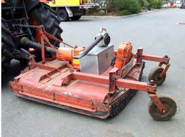
Machinery hygiene – the blower is carried on slasher deck for cleaning in field
