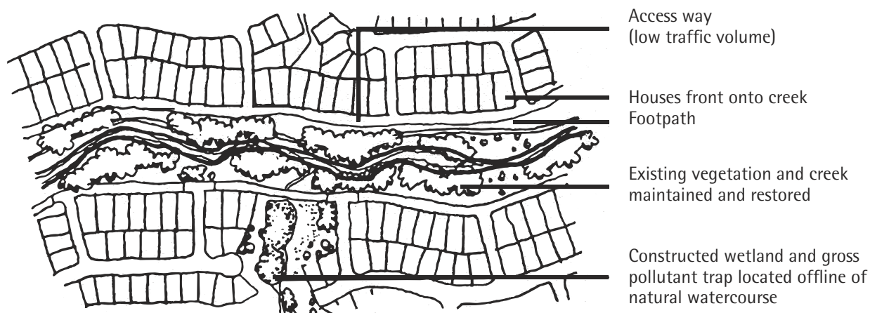
Figure 3. Protecting the natural creekline (Source: NSW EPA 1996)
