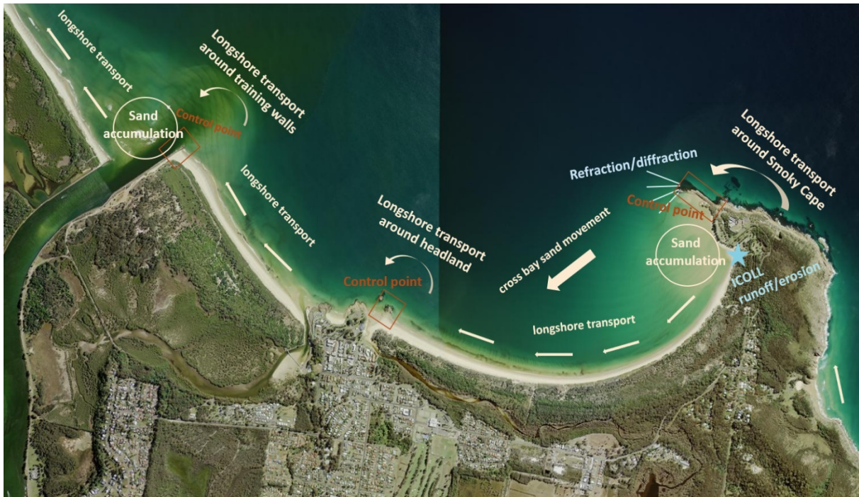
Figure 3 Conceptual model of Trial Bay coastal processes. Alluvium Consulting (2021).
