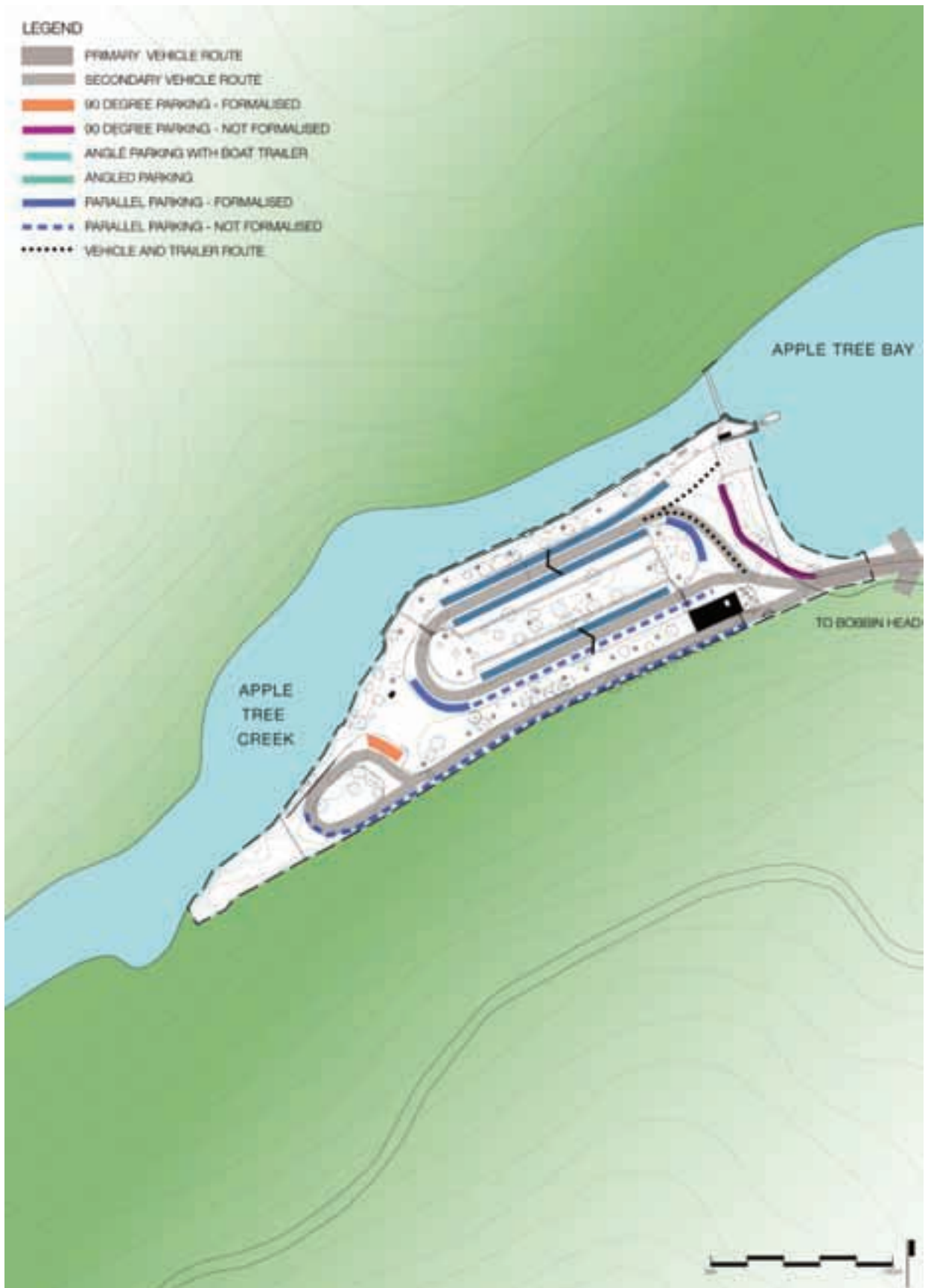
Figure 4.6: Existing Vehicular Circulation and Parking
