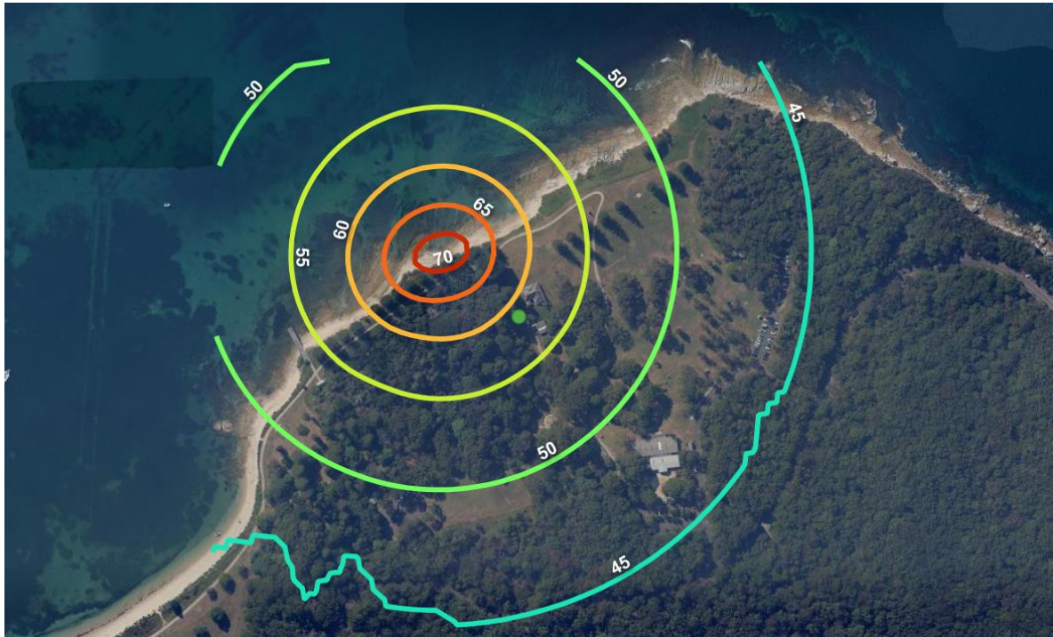
Figure 11 Noise contours of concreting conducted along the North-West foreshore
