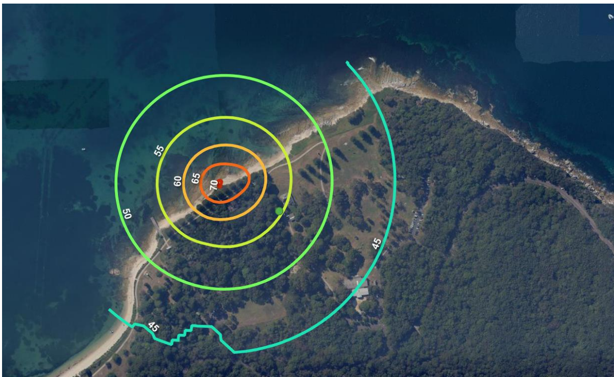
Figure 12 Noise contours of general construction conducted along the North-West foreshore
