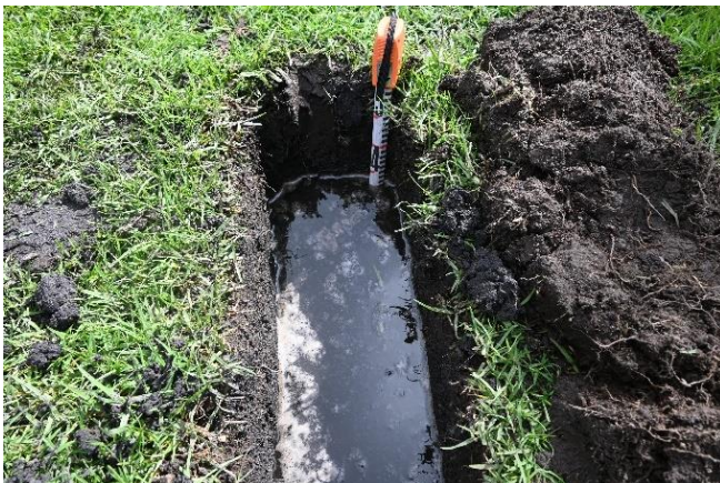
Figure 80. TP1, end of excavation, north section, example of ground water seepage
