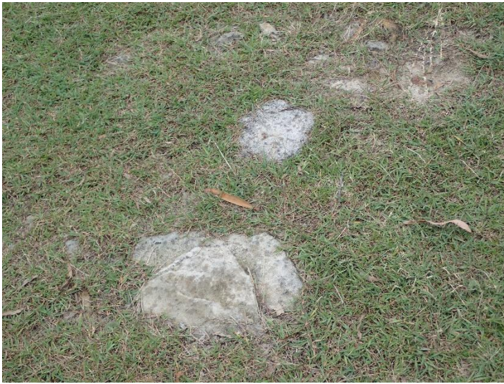
Figure 52. Sandstone fragments in the fill of the building pad adjacent to the visitor centre.
