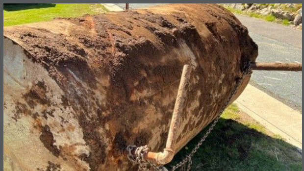
A decommissioned underground diesel tank. Image: A Clifford / DCCEEW
