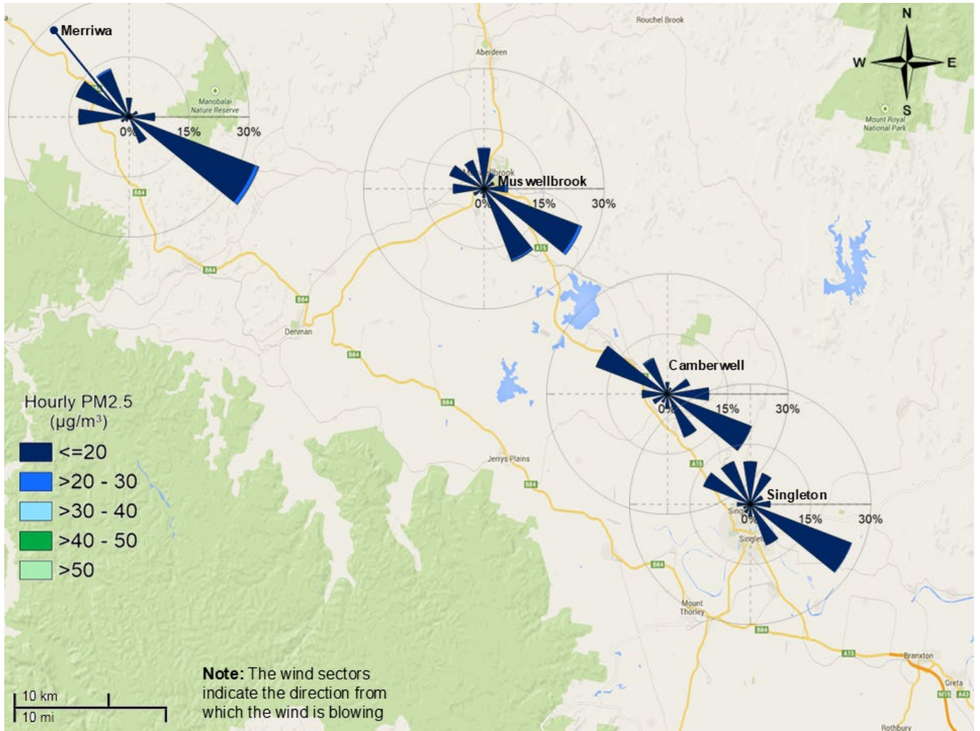
Figure 5 Hourly PM2.5 pollution rose map for the Upper Hunter region for spring 2023
