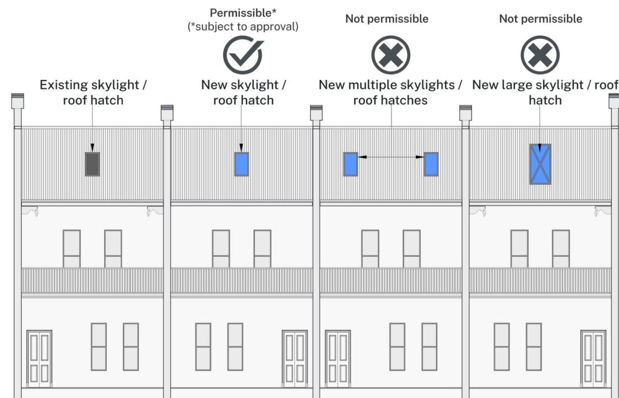
Figure 7 Group of terraces – roof penetrations on rear elevations
