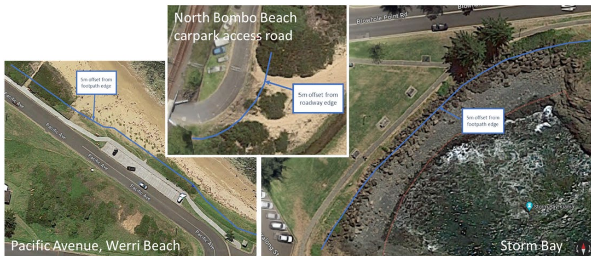
Figure 13 Approximate locations of erosion scarp to reach trigger and threshold (to be confirmed through REF and approvals process) (Source: Google, Kiama coastal CMP 2024).
