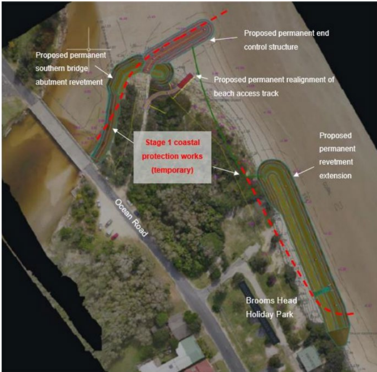
Figure 15 Proposed revetment extension and temporary (stage 1) works to be implemented as part of the Brooms Head coastal erosion mitigation strategy
