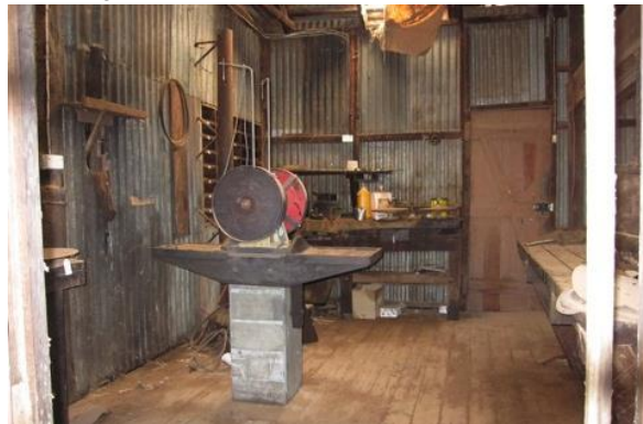
Shear sharpening area in Engine Room
